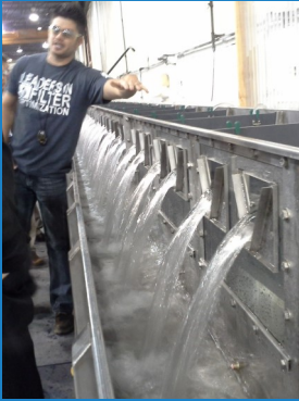
AWI can provide a shop performance test to prove perfect flow distribution.
