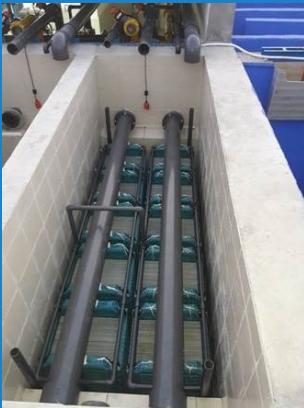
This 7' x 16' tank can treat up to 1 MGD!
