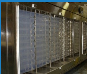
The tube sheets lift out of the unit for easy bulb changing and maintenance.
