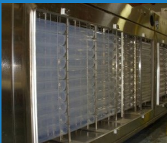
The UV lamps irradiate from outside the AFP tubes.
