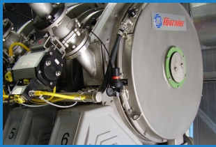
Sludge is fed at low pressure into the channel and rotates between two parallel revolving stainless steel revolving elements.
