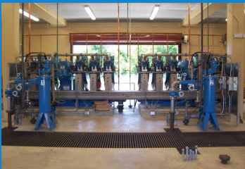
The Rotary Press is a clean and simple dewatering system.
