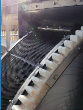
The drive mechanism is a nylon pinion, which engages with a gear ring on the outside of the drum.
